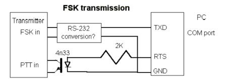
What goes in the "RS-232 conversion" box depends on your transmitter's FSK input. Odds are, it can be exactly the same as the circuit shown for the PTT connect: use an opto-isolator with a series resistor to convert the RS-232 levels to open/close keying.
