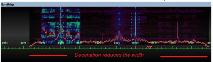
SoftRock on K2 IF tuned to 10MHz WWV. The sound board is set to 48K sample/second.
