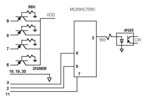
As an alternative to the LPT connection, the keyer can be wired to a serial port as shown. The serial port connection requires a 5V power supply, and requires an RS-232 to 5V level conversion:
