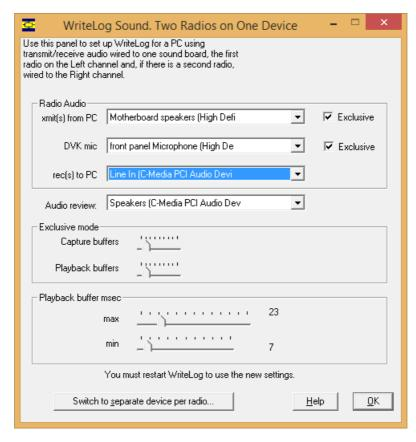
This is the setup for a shack cabled for one rig, or for two rigs using Y cables with the L/R channels on a single sound board input for receivers and single sound board output for transmitters.
