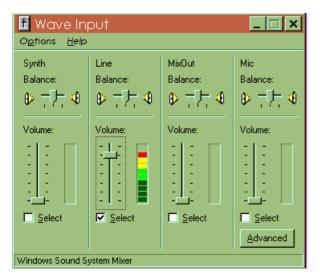
If you want to see the display with the color coded level meters as shown here, then you need to be running RttyRite in receive mode (or run the Windows Sound Recorder and press its Record button). You want to not see any red indicators as shown in this picture. That means the receiver audio is overloading the sound board's receive input. Lower the slider position until you see only green and yellow peaks.
