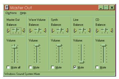
The "Wave Volume" control is the one that controls the AFSK output level (and so does the Master Out). Don't overlook the
