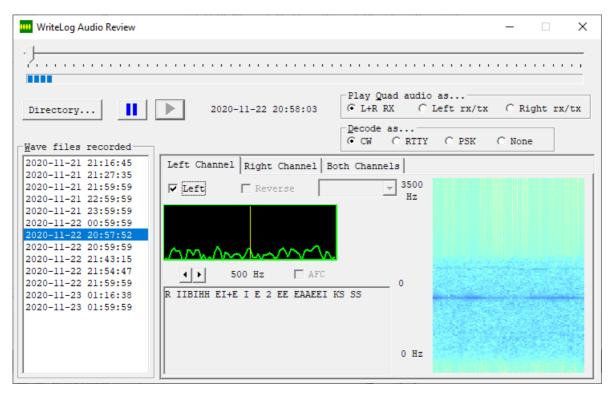
The Play Quad Audio as... buttons are enabled only if the original recording was done with four channels.
