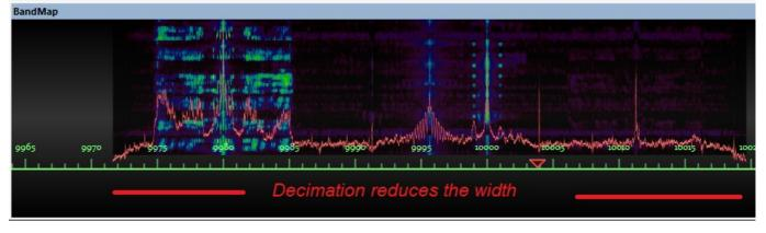
SoftRock on K2 IF tuned to 10MHz WWV. The sound board is set to 48K sample/second.
