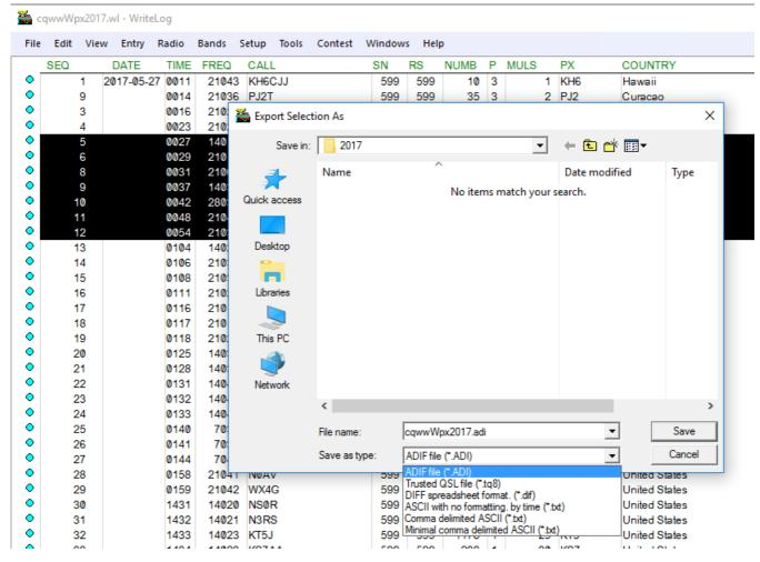
The Save-As-Type box on the file selector controls the file format.
