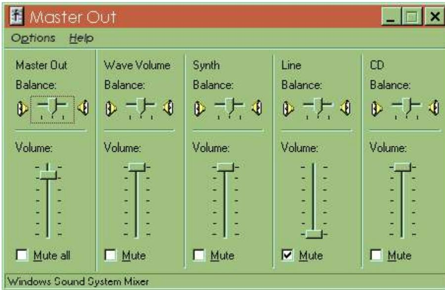
The "Wave Volume" control is the one that controls the AFSK output level (and so does the Master Out). Don't overlook the other controls! Be sure to turn off the Line control—that is the Line *in* and the audio from your rig. You don't want it tripping your VOX. To set the receive levels, use the Options Properties menu command and you get this dialog:
