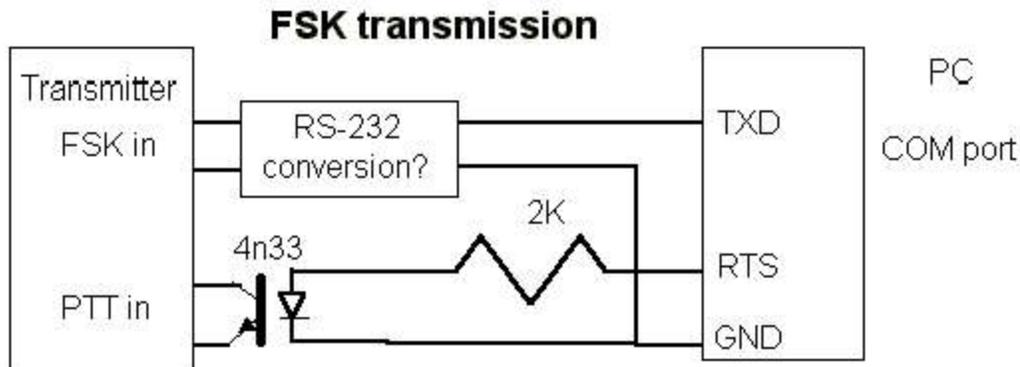
What goes in the "RS-232 conversion" box depends on your transmitter's FSK input. Odds are, it can be exactly the same as the circuit shown for the PTT connect: use an opto-isolator with a series resistor to convert the RS-232 levels to open/close keying.
