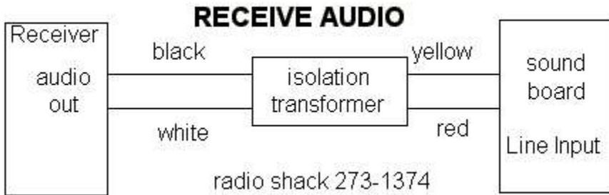
While the isolation transformer is optional, it is highly recommended as a precaution against introducing ground loops that get 60Hz hum into the signal. With this connection, you have enough to do receive only RTTY.
