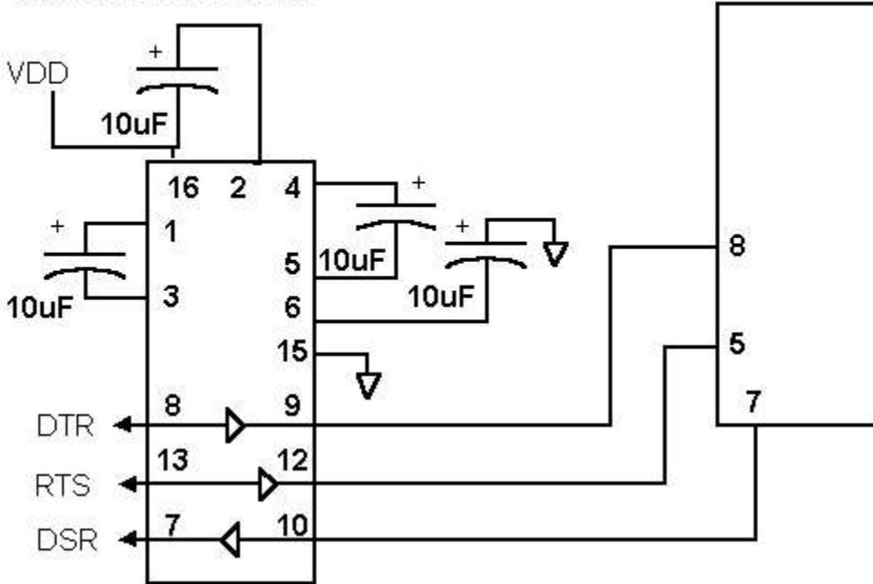
Finally, the keyer chip can be wired for several control functions. Any of these can be omitted or used as desired by the builder:
