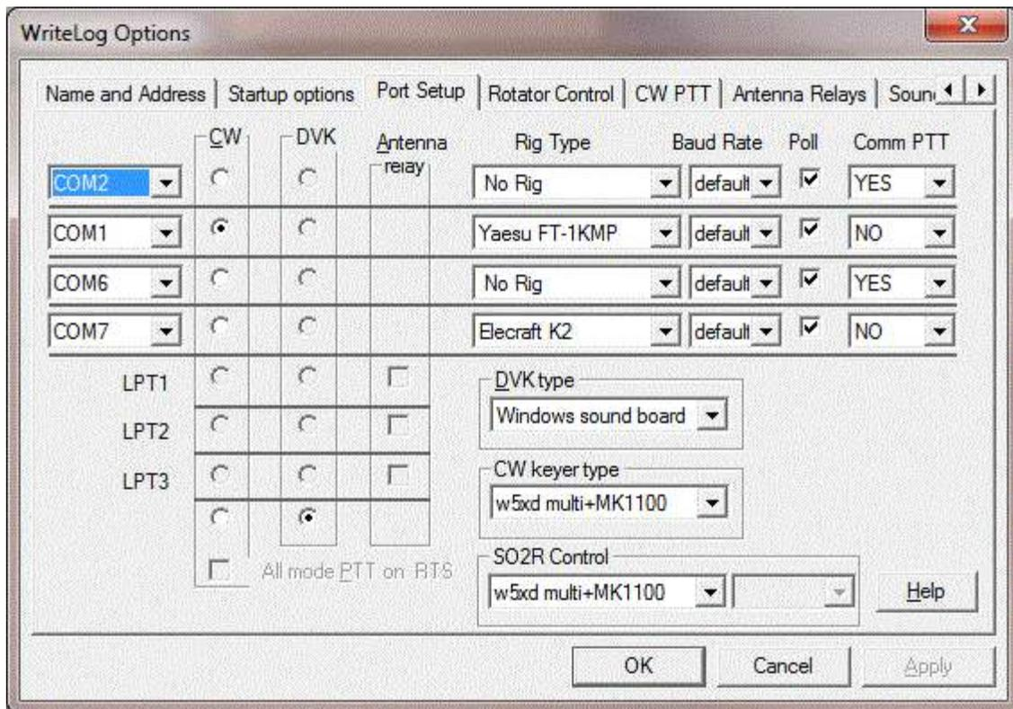
You may select any number of rigs to be controlled, and any number of antenna relays to be controlled, but only one CW output and only one DVK output.
