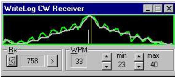
The WriteLog CW Receiver screen automatically appears when you select the CW mode. The frequency display is the top left panel. It always displays the frequency ranges +/- 250Hz from a center frequency shown by the light blue vertical bar in the very. The yellow vertical bar shows your receive frequency. You can set the center (transmit) frequency in WRITELOG.INI using the CW\_XMIT\_FREQ setting.
