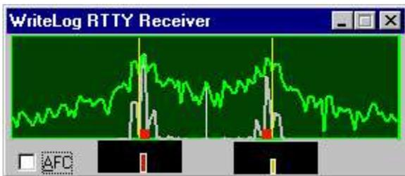
The picture is 500Hz wide and the two yellow vertical lines show you the mark and space tones. The space tone is on the left (lower frequency) and the mark is on the right unless you select FSK Reverse. The two red boxes show the frequencies of the loudest tones being received.
