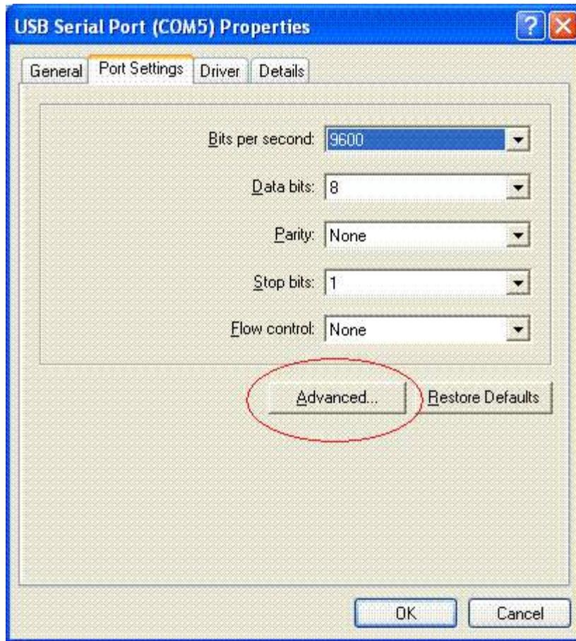
In this dialog, you can set the "Latency timer" to 1msec on this device. 60WPM RTTY has timings of about 22msec, so a 1msec latency could cause the desired 22msec to vary +/- 1 msec, which is acceptable to most RTTY decoders. However, the 16msec default latency setting for this hardware causes timing errors that prevent decoding in many cases.
