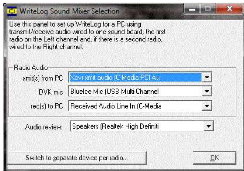
This is the traditional setup for a shack cabled for one or two receivers with their transmitters as L/R channels into a single sound board input and single sound board output.
