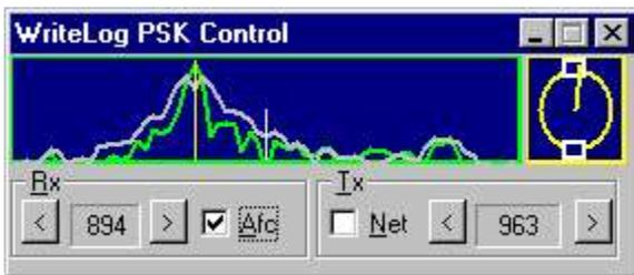
The WriteLog PSK Control screen automatically appears when you select the PSK modes. The frequency display is the top left panel. It always displays the frequency ranges +/- 250Hz from your transmit frequency. The light blue vertical bar in the very center is your transmit frequency. The yellow vertical bar shows your receive frequency.
