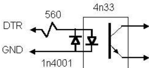
WriteLog also puts the PTT signal on the RTS line of the same comm port. WriteLog allows you to use the same COMM port for both CW and for rig control, but you will have to build your own Y cable that sends the appropriate wires (TXD, RXD) to the rig control port and the appropriate wires (DTR, RTS) to your CW and PTT circuits.
