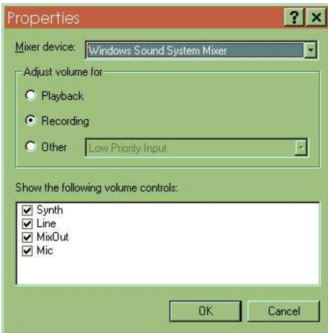
Click the "Recording" button under "Adjust volume for" and turn on the "Line" (or "Mic") buttons and click OK. You get the next picture:
