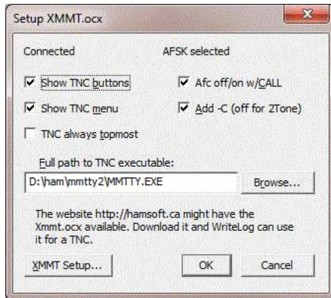
The critical setting is the "Full path to TNC executable". Use the Browse... button to select the MMTTY.EXE (or compatible) TNC program. If you intend to run more than one of these TNCs concurrently (either for multiple radios, or for cloned views on the same sound board channel) then duplicate the MMTTY.exe into multiple folders, and use this menu entry on each of the RttyRite windows to browse to one in a different folder.
